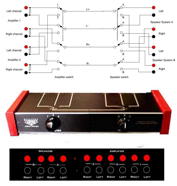
Top – A 3-amplifier to 3-speaker systems SP 1. Functional wiring diagram is shown on top of chassis. Bottom – Rear panel layout of a 3 to 2 SP 1
