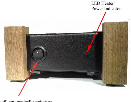
On Switch (High Voltage will automatically switch on after 20 seconds)
