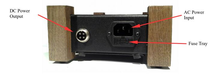
The power supply is connected to the amplifier chassis with the supplied power interconnect cord. Never power on the power supply without making this connection. The two chassis may be stacked or separated as permitted by the power interconnect cord.
